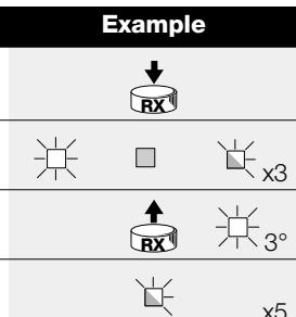
**N.B.:** if the procedure was performed correctly, the Led will flash 5 times after a few moments.
